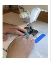
Step 7: Topstitch 1/8" from each long edge of the tab. You want to stop this stitch line where it will intersect with the topstitch you will do around the design area of the connector. Repeat for all your connectors.
